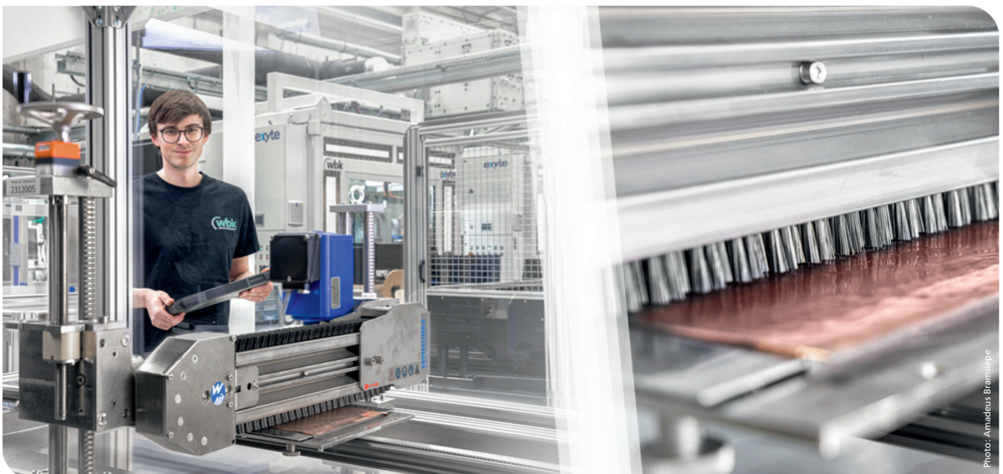
Experimental setup for the direct recycling of battery electrodes through utilization of a sword brush.
