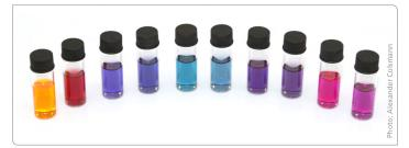
KIT has invented highly specialized and eco-friendly organic semiconductor inks for the fabrication of organic solar cells from water or alcohol instead of toxic aromatic solvents.
